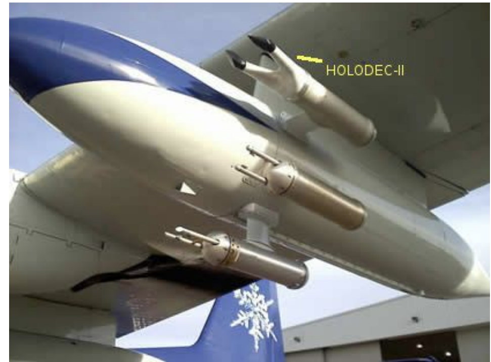
HOLODEC-II installed on C-130
